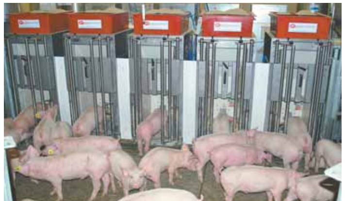
Precision feeding system fattens hogs at less cost with less waste, by changing the amount of protein and lysine each animal gets.
