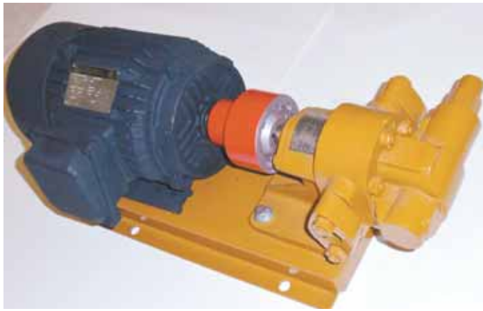
Steve Chastain makes his own portable transfer pumps using both off-the-shelf components and parts he casts himself. Photo above shows an electric-powered pump.
