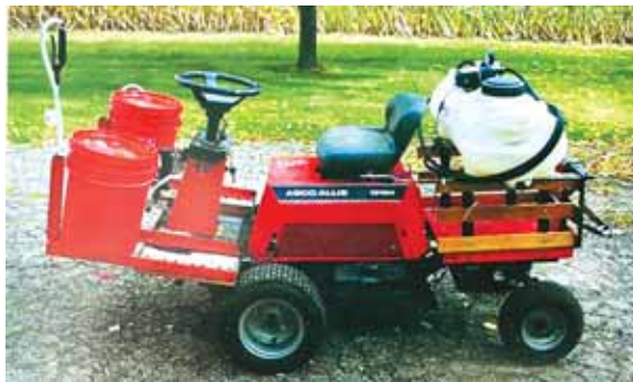
Denny Michels converted an old riding lawnmower into a handy spray rig that he uses around his campground.
