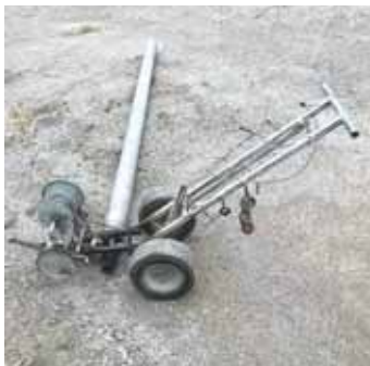
Vandevetter used a leftover piece a 4 1/2-in. aluminum alloy pipe for his roller.
