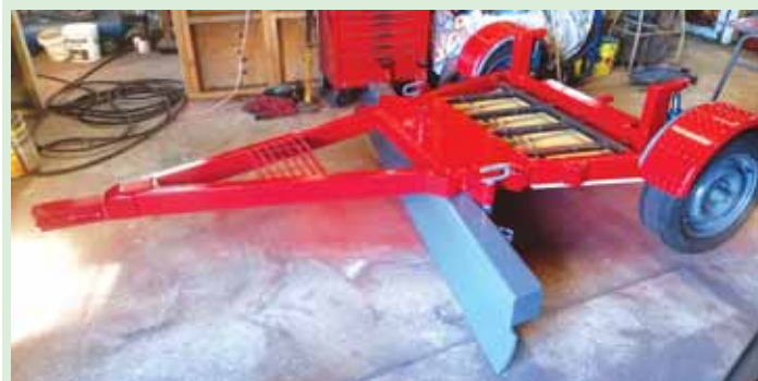
Gunn filled the tires with water for smooth grading. He added more weight by filling the space in the chassis between the bridge and the back end with concrete.
